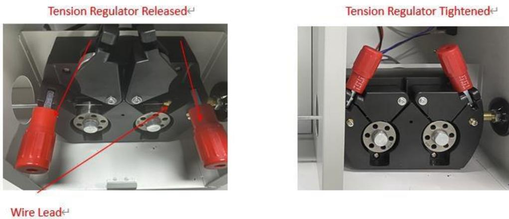
4. Connect the interface of wire tube; Press Manual Feeding in the panel to feed wire to the tube in the interface; Fix the wire feeding inlet onto the wire feeding mechanism; Tighten it by bolt.
