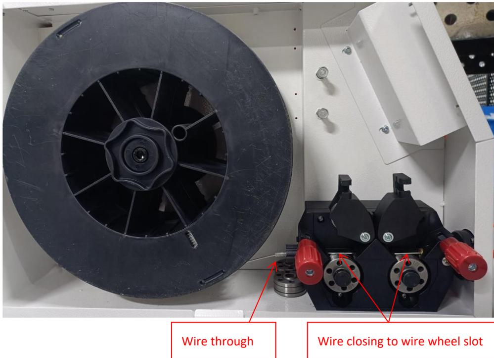
**Internal structure of wire feeder**
