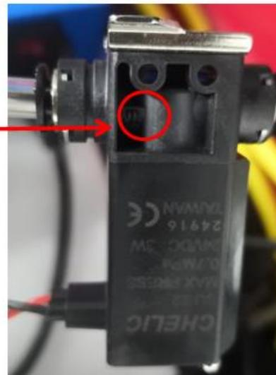
**Gas valve ±:** control switch of protective gas.
